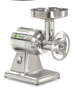
Polished aluminium structure with S.S. hopper - Machine with a completely removable grinding unit that allows it to be placed in the refrigerator without having to remove minced meat residues after each use in accordance with the HACCP hygiene standards - the grinding unit in S.S. AISI 304 can be washed in the dishwasher - low voltage controls - meat inlet ø 52 mm - oiled gear motor.
